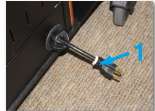
1. Pull out the retractable power-cord located at the lower right side on the back of the cart and plug it into a power source.
