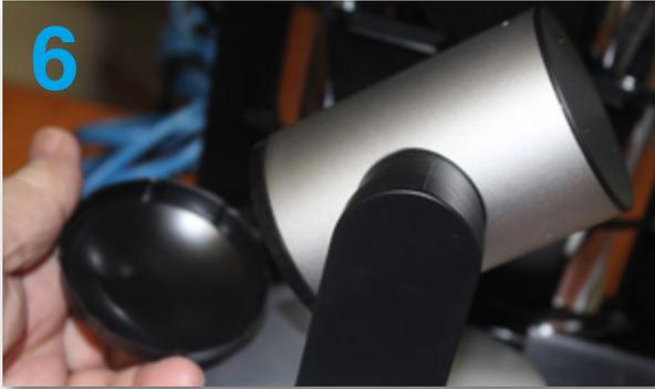
6. The Webcam has a lens cover, simply slip the cover off the lens opening end and store it on the opposite end of the camera while the camera is in use. The camera will move on its own during computer system powering on and off so some movement of the camera is normal.
