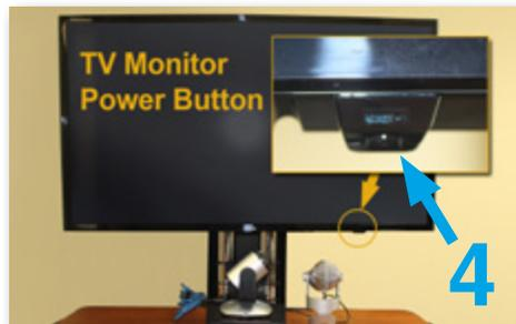
4. Locate the power button for the TV monitor on the bottom edge and turn on the power for the monitor.
