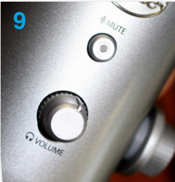
9. The microphone controls on the top side include the Mute button (also status light) and the headphone volume control. The microphone is muted when the mute button is depressed and the light is blinking. The headphone volume control ONLY adjusts the output volume to the headphone output jack and to headphones if plugged in and in use.
