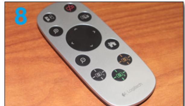
8. The webcam remote controls pan/tilt movement, zooming, it can have 3 preset for zoom/tilt/pan, mirror (flip) the image horizontally and has a camera off button. See a copy of the operation instructions below.
