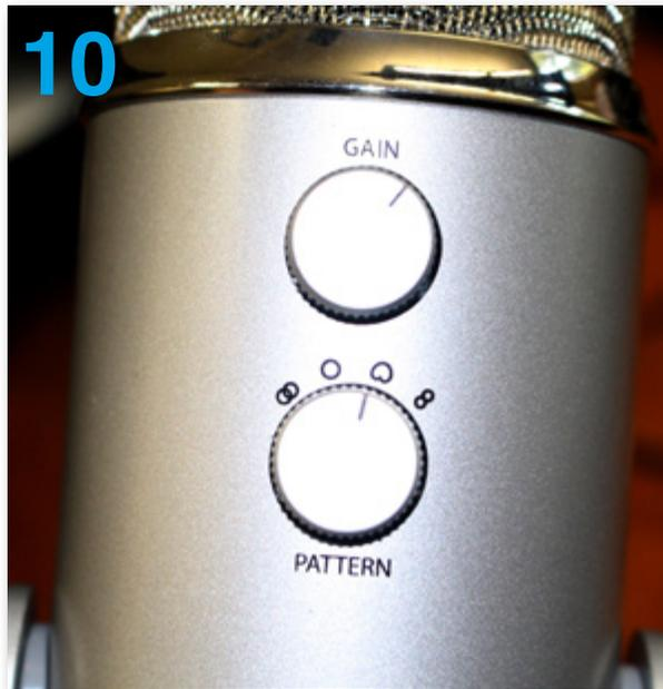
10. The microphone controls on the underside include the gain controls and the pattern selection control. The gain adjusts the sensitivity of the microphone (how well it picks up sound) too much gain can cause distortion. The pattern selector allows you to select the pickup pattern for the microphone, see the instruction below for more details.
